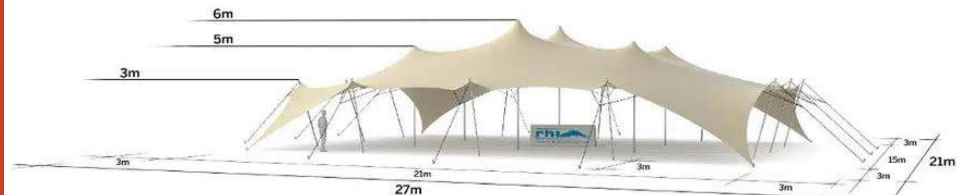
Corner on ground configuration
